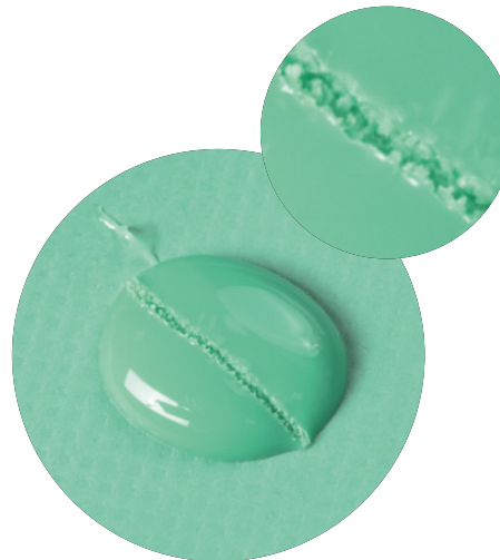
Fig. 35: Absence of an unpolymerized layer (smear layer) shows compatibility of the used materials.
